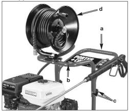
3. Connect wand to gun. Tighten securely.
